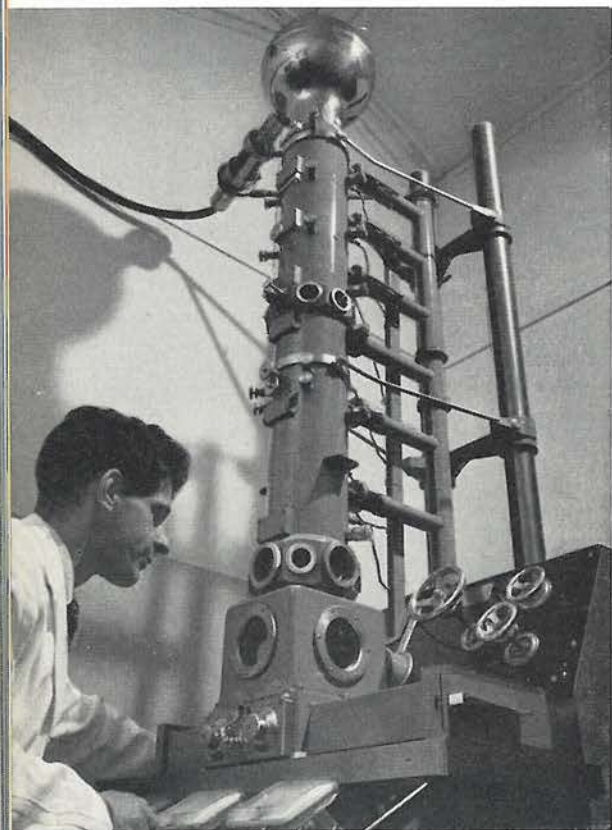
An electron diffraction camera designed and built in the workshops of the Chemical Research Laboratories.
