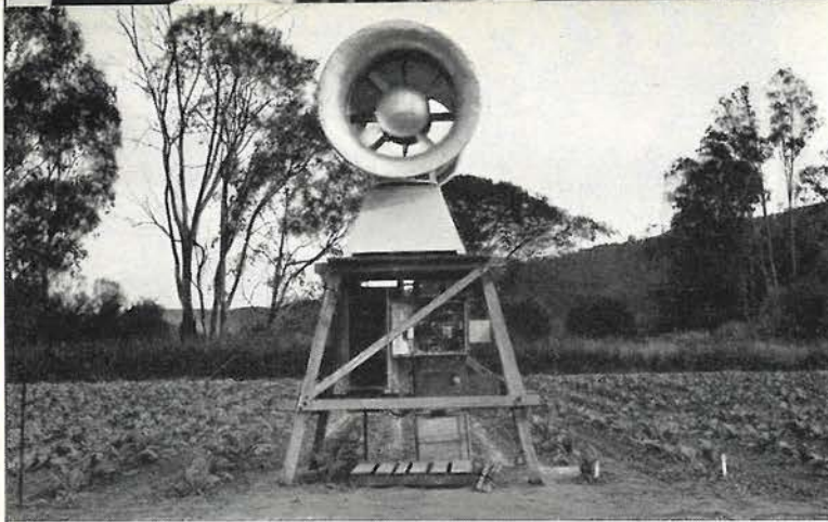
↑ Experiment in forced ventilation of tobacco crop for prevention of blue mould.
